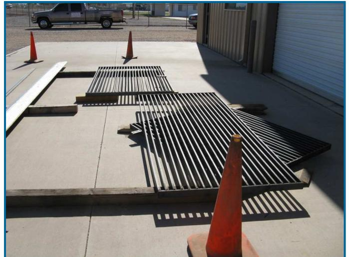
**Figure 6:** Grates like these are used to isolate 14-inch amurs, which cannot pass between the 1-3/4” openings.
